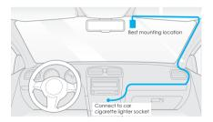
3) Wipe clean the installation surface of the windscreen with a dry cloth, it must be grease free for the sticky pad to stick firmly.4) Peel the protection film off the sticky pad and camera lens.
