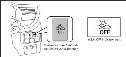
A.S.A. OFF indicator light will illuminate at the meter panel. Every time you start the engine by the engine switch operation, A.S.A. function will return to ready state.
