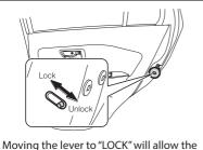
Moving the lever to "LOCK" will allow the door to be openned only from the outside.
