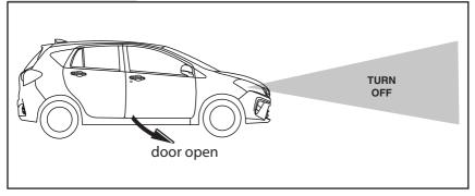
The headlights are automatically turned off if the driver's door opened after the engine switch is turned to "OFF" or "ACC".
