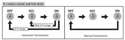
When brake pedal is not depressed, pressing the Push Start/Stop Button will change the engine mode.
