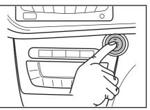
③ Push the Push Start/Stop Button within 4 seconds after the buzzer sounds and the engine switch indicator turns green.
