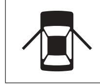
Door ajar warning light turns on when the driver's door is closed and does not turn on when the driver's door is opened.
