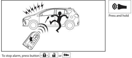
The alarm will sound for 45 seconds if any of these buttons are not pressed.
