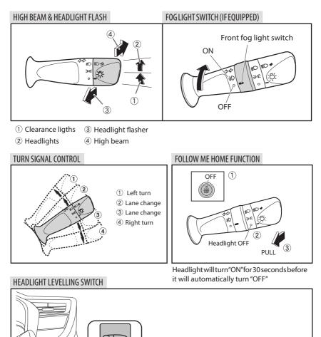
Rotate the dial up & down to change the direction.
