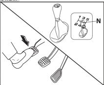
**For MT**: Move the gear shift to 'N' while depressing the clutch pedal
