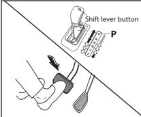
① **For AT** : Move the gear shift to 'P' while depressing the brake pedal.
