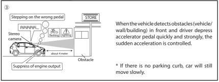
If the depression of accelerator pedal is strong but not quick at under 4km/h, only warning is operated.
