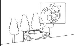
② Vehicle retains brake force for 2 seconds
