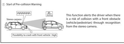
This funtion are operates when speed are about 4~30 km/h
