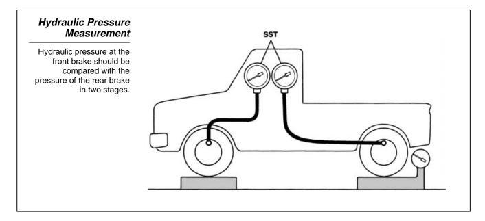
Next, the hydraulic pressure at the front brake should be compared with the pressure of the rear brake in two or three stages as specified in the Repair Manual.
