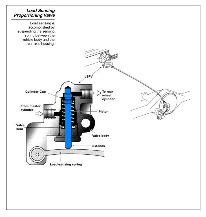
LSPV Operation As a vehicle is loaded, the leaf springs are compressed as the vehicle body lowers. The load sensing spring provides a variable force pushing the proportioning piston up as the vehicle is loaded. As the piston is lifted, a higher brake hydraulic pressure is required to force the piston down resulting in higher pressure at the rear wheels.
