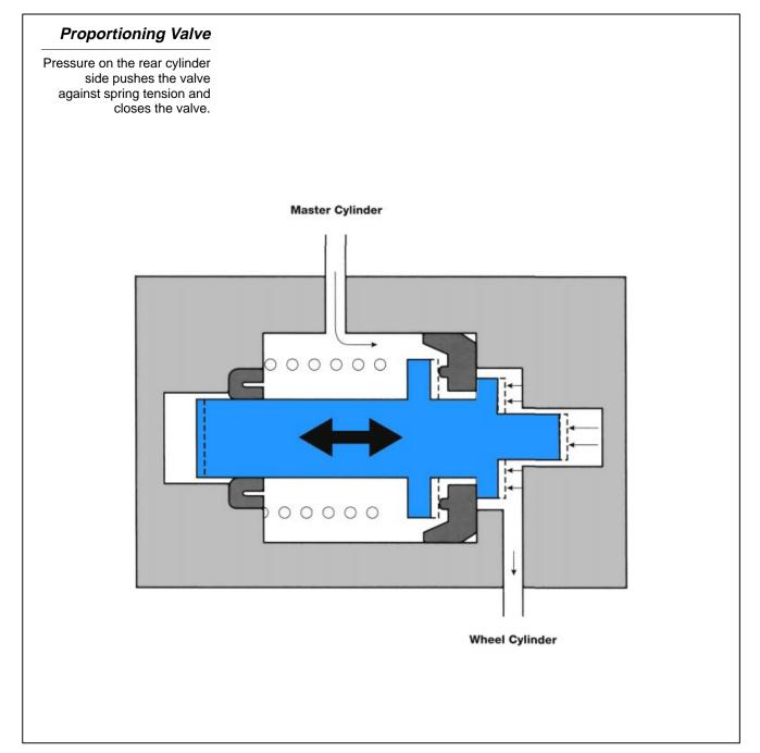
In order to release the pressure between the proportioning valve and the rear wheel cylinders, the valve seat floats as shown in the illustration. When the pressure from the master cylinder is released, the pressure difference on the valve seat causes it to be pushed away from its seated position on the valve body. This allows fluid to pass the valve seat and the brakes to release.
