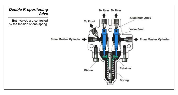
The movement of both valves is controlled by the tension of one spring. With a single spring, a balanced pressure is applied to each valve through the retainer.
