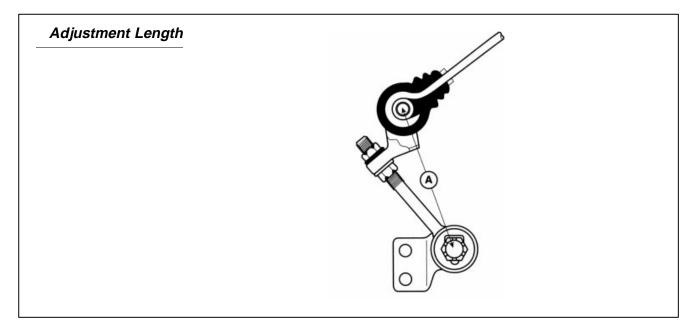
If distance (A) is too short, the hydraulic pressure breaking point will decrease. Hydraulic pressure to the rear wheel cylinders will be lower than normal, reducing braking performance.
