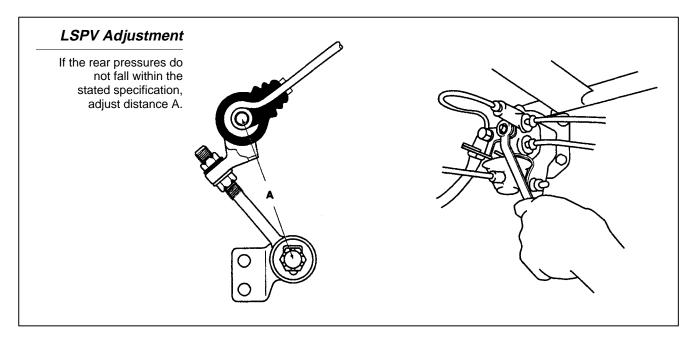
If adjustment of the springs does not bring the rear pressure into specification, adjust the valve body:
