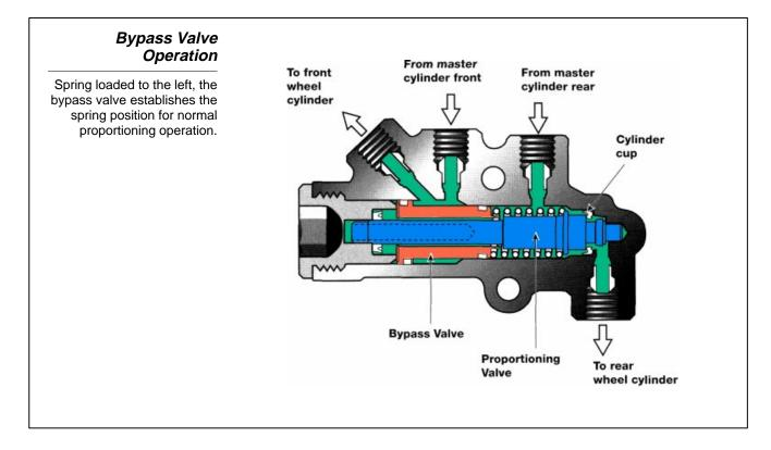
Should the hydraulic circuit to the front brakes fail, rear brake pressure will move the bypass valve to the right, forcing the proportioning valve to the right, which allows unregulated pressure to apply the rear brakes.
