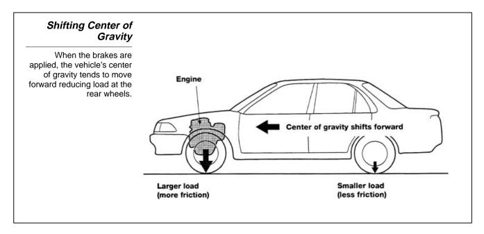
Assuming that the front and rear wheels exert an identical braking force in the above condition, the rear tires, which are subject to a smaller load, tend to lockup early. This will cause the rear tires to lose traction or skid.
