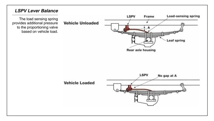
Rear wheel cylinder pressure is adjusted according to increases or decreases in vehicle load. The pressure change for one rear wheel is shown below.
