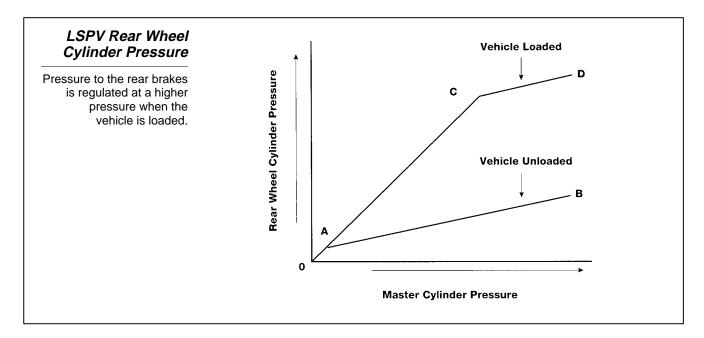
Unloaded Vehicle When unloaded, *a* vehicle body rises to normal vehicle height and no force from the load sensing spring is applied to the piston. The rear wheel cylinder is regulated at a lower pressure as shown by the line O - A - B in the chart on the previous page.
