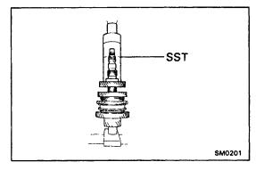
(f) Using SST and a press, install the 3rd driven gear. SST 09316 – 60010 (09316 – 00010)
