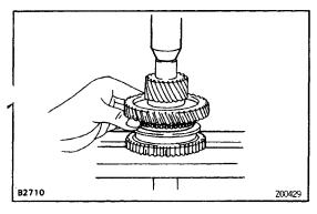
(d) Using a press, install the 1st gear and No. 1 hub sleeve.
