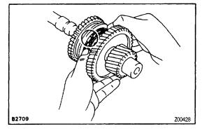
(c) Place the synchronizer ring on the gear and align the ring slots with the shifting keys.
