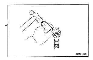
(c) Using a screwdriver and hammer, drive out the thrust washer.
