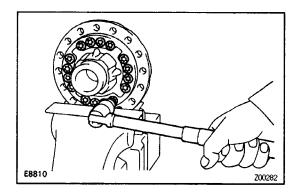
(b) Using a torx wrench, remove the sixteen torx screws. Torx wrench: T50 09042–00040
