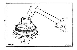
(i) Using a plastic hammer, carefully tap the differential case to install it.
