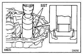
(e) Using SST and a press, install the taper roller bearing. SST 09316–60010 (09316–00010, 09316–00040)
