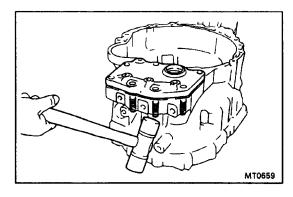
(b) Using a plastic hammer, tap the stud bolt and remove the transaxle case cover.
