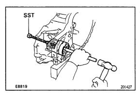
(d) Using a SST, brass bar and hammer, remove the taper roller bearing outer race. SST 09612–65014
