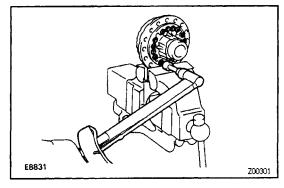
(j) Using a torx wrench, install and torque the sixteen torx screws.
