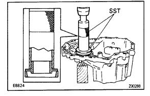
(f) Using SST and a press, install the taper roller bearing outer race.
