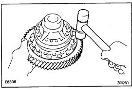
(c) Using a plastic hammer, tap out the ring gear.
