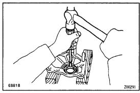
(c) Using a screwdriver and hammer, drive out the oil seal.
