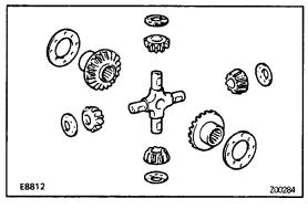
(e) Remove the two differential side gears, two side gear thrust washers, differential pinions and four pinion washers from the differential left case.
