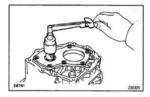
(c) Using a small torque wrench, measure the preload.
