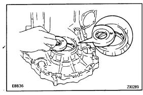
(g) Install the transmission oil baffle.
