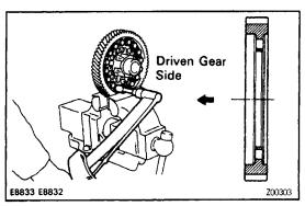
HINT: Align the matchmarks on the differential left case and contact the ring gear.
