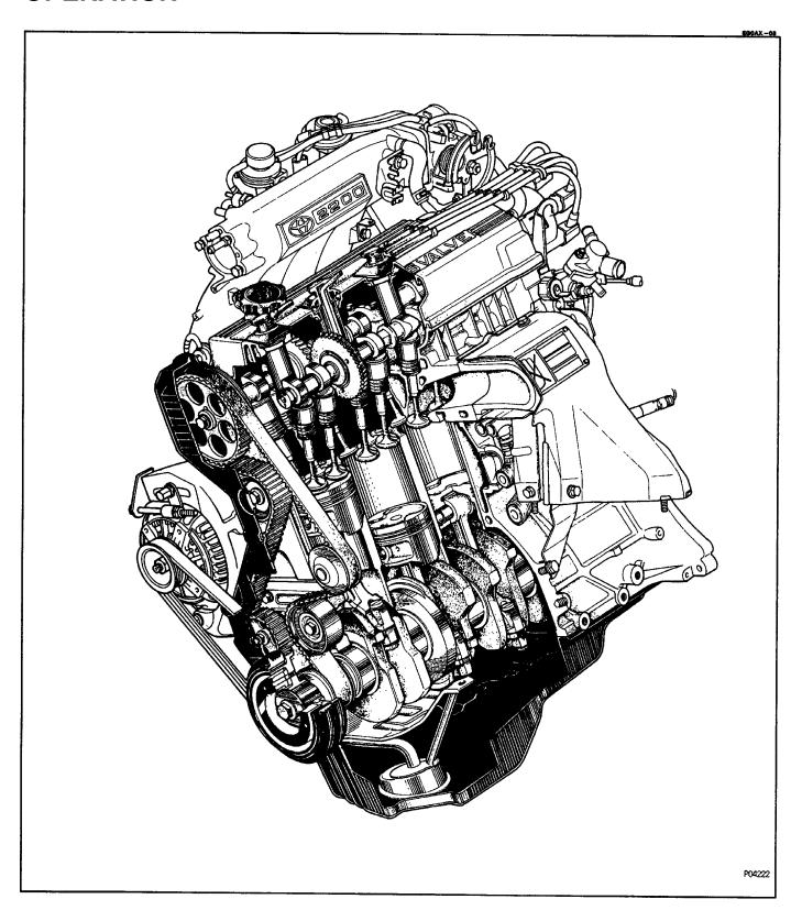
The 5S–FE engine is an in–line, 4–cylinder engine with the cylinders numbered 1-2-3-4 from the front. The crankshaft is supported by 5 bearings inside the crankcase. These bearings are made of aluminum alloy.
