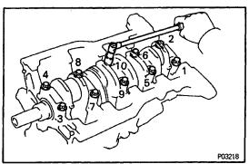
(i) Remove the main bearing caps. (See procedure (a) and (b) above)
