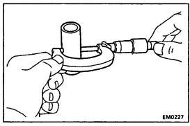
(b) Using a micrometer, measure the piston pin diameter.
