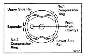
(b) Using a piston ring expander, install the two compression rings with the code mark facing upward. Code mark:
