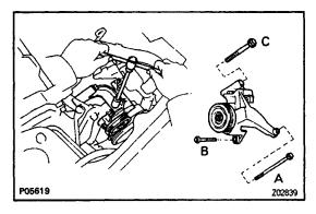
(b) Install the idler pulley bracket with the three bolts.
