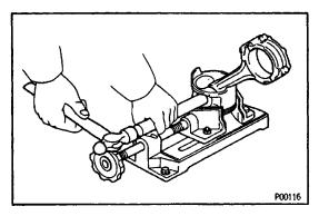
(c) Using plastic–faced hammer and brass bar, lightly tap out the piston pin and remove the connecting rod.
