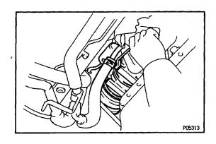
(d) Tighten the two bolts of the lower side of the A/C compressor.
