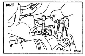
(b) Tighten the two bolts holding the clutch release cylinder to the transaxle.
