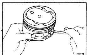
(b) Using a groove cleaning tool or broken ring, clean the piston ring grooves.
