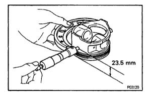
(a) Using a micrometer, measure the piston diameter at ring angles to the piston pin center line, 23.5 mm (0.925 in.) from the piston head.
