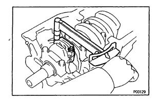
(h) Install the connecting rod cap.(See step 6 in Cylinder Block Assembly)
