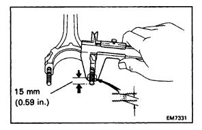
(b) If the cap nut cannot be turned easily, measure the outside diameter— of the connecting rod bolt with a vernier caliper.
