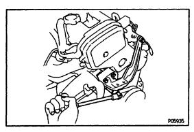
5. REMOVE RH ENGINE MOUNTING BRACKET
