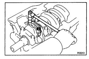
(i) Remove the connecting rod cap.
