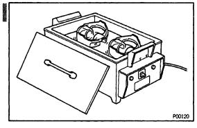
(b) Gradually heat the piston to  $80 - 90^{\circ}$ C ( $176 - 194^{\circ}$ F).
