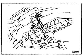
30. REMOVE REAR ENGINE MOUNTING BRACKET
