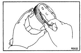
(b) Remove the two side rails and oil ring by hand. HINT: Arrange the piston rings in correct order only.
