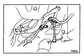
(i) Install the parking brake cable with the two clamps and three bolts.
