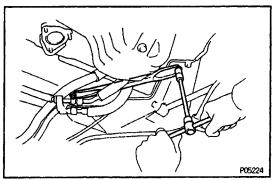
(h) Install the lower suspension brace with the two bolts.
