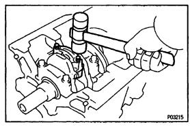
(c) Using a plastic–faced hammer, lightly tap the connecting rod bolts and lift off the connecting rod cap.HINT: Keep the lower bearing inserted with the connecting rod cap.
