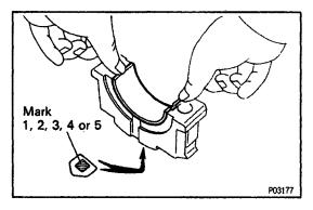
(b) Align the bearing claw with the claw groove of the main bearing cap, and push in the five lower bearings.HINT: A number is marked on each main bearing cap to indicate the installation position.
