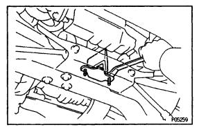
(e) Install the damper with the two bolts.
