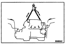
(c) Keep the engine level, and align RH and LH mountings with the body mountings.
