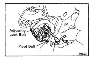
(c) Remove the pivot bolt and adjusting lock bolt, and disconnect the alternator from the bracket.
