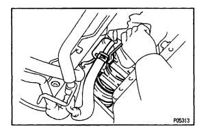
(h) Remove the two bolts, and disconnect the A/C compressor from the engine.
