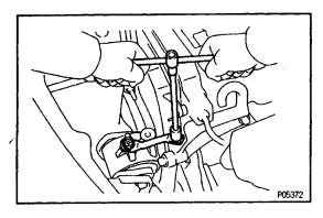
(f) Attach the LH mounting insulator to the body, and temporarily install the through bolt.
