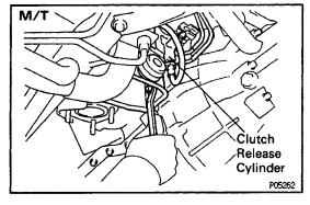
(b) Remove the two bolts and mounting bracket, and disconnect the clutch release cylinder from the transaxle.
