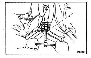
(g) Install the A/C pipes with the two clamps and nut.
