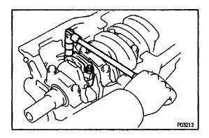
(b) Remove the connecting rod cap nuts.
