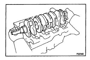
(c) Lift out the crankshaft.
