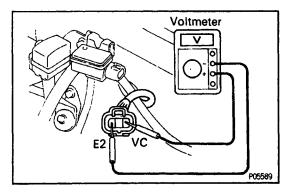
(c) Using a voltmeter, measure the voltage between connector terminals VC and E2 of the wiring harness side.
