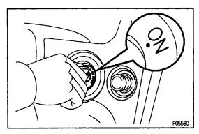
(b) Turn the ignition switch ON.
