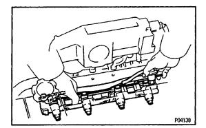
2. REMOVE DELIVERY PIPE ASSEMBLY (See step 2 to 9 in Injectors Removal)
