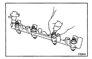
**2. INSTALL INJECTOR COVER TO DELIVERY PIPE** (a) Install a new insulator to each injector.
