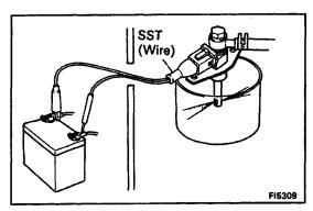
(h) Connect the test probes of the SST (wire) to the battery, and check that the fuel spray is as shown. SST 09842–30050
