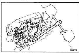
3. INSTALL THROTTLE BODY (See Throttle Body Installation)
