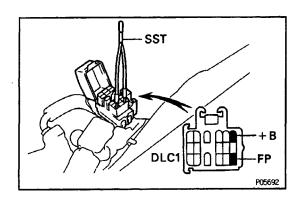
(e) Using SST, connect terminals +B and FP of the data link connector.
