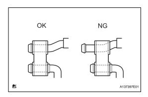
(c) Check the No. 4 exhaust pipe supports.
