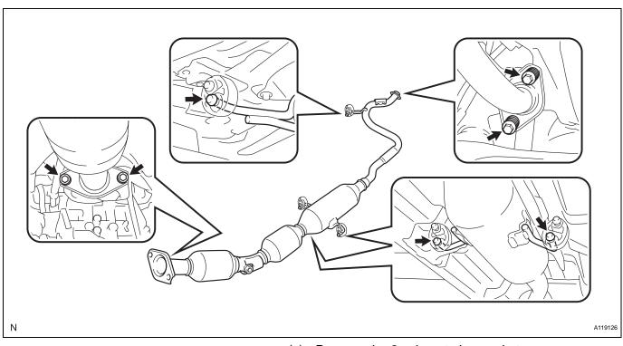
(c) Remove the 2 exhaust pipe gaskets.
