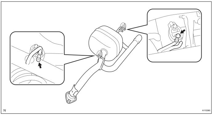
(b) Remove the 3 No. 4 exhaust pipe supports and the exhaust tail pipe assembly. (for Sedan)
