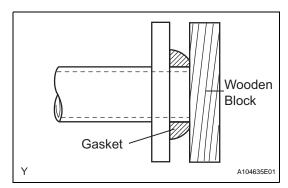
(b) Using a plastic hammer and a wooden block, tap in a new exhaust pipe gasket until its surface is flush with the exhaust manifold.
