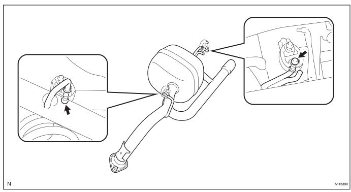
(b) Install the 3 No. 4 exhaust pipe supports and the exhaust tail pipe assembly. (for Sedan)
